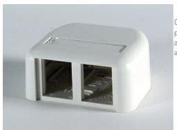
Ortronics TracJack Surface Mount Outlet Boxes accept front-loading TracJack modules and provide snap-on covers and snap-in label fields. Boxes are supplied with screws and double-sided adhesive tape for mounting onto almost any surface Meet UL2043 and are suitable for installation in air handling spaces (ie plenum spaces)
