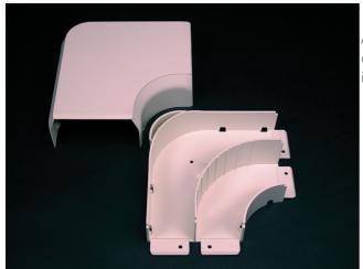
A 90 degree flat corner with integral dividers to provide 2'' (51mm) cable bend radius for UTP and fiber optic installations. Ideal for layin or pull-through installations.
