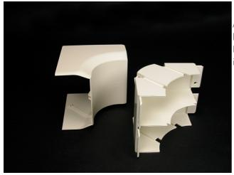
A 90 degree internal corner with integral dividers to provide 2" (51mm) cable bend radius for UTP and fiber optic installations. Each leg is 4 1/2" (114mm). Ideal for lay-in or pull-through installations.
