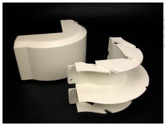
A 90 degree external corner with integral dividers to provide 2" (51mm) cable bend radius for UTP and fiber optic installations. Each leg is 4 1/2" (114mm). Ideal for lay-in or pull-through installations.
