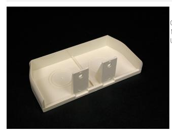
Closes off raceway end runs. Can be used to feed raceway using 1/2'' or 3/4'' trade size conduit. Holes for conduit must be drilled. Use a step drill or other means.
