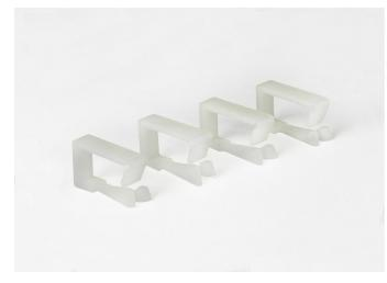
Nonmetallic clips snap into tabs in preset base. Hold up to one meter of cable. Maintain 1 1/4"" (32mm) bend radius. Four clips included in kit.
