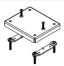
Blank plate for abandoning preset or can be field punched for custom sized opening. Flush plate is 3.7/8" x 4.5/8" (98mm x 117mm).
