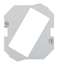
Device Mounting Plate - device plate that will accept Decorator style devices such as 20A receptacles, GFCIs, 106 adapters or A/V devices. Designed to fit into two (2) gangs of the 4AT Series Poke-Thru.
