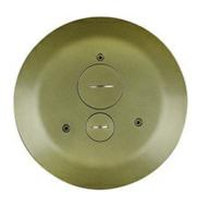
Complete with one-piece finish flange and conduit assembly. Conduit assembly consists of one 3/4inch trade size conduit and one 1 1/2inch trade size conduit. Finish cover flange provided with one 3/4inch trade size screw plug opening and one 1 1/2inch trade size screw plug opening. Covers available in painted black (BK), gray (GY), brass (BS), bronze (BZ), and brushed aluminum (AL). NOTE: Assembled with scrub water gasket. For use on tile, wood or carpet floors.
