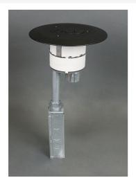
Complete with one-piece finish flange and conduit assembly. Conduit assembly consists of one 3/4" trade size conduit and one 1 1/2" trade size conduit. Finish cover flange provided with one 3/4" and one 1 1/2" trade size screw plug opening.
