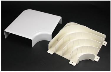
For right angle turns on the same surface. Integral dividers provide 2'' (51mm) cable bend raduis for UTP and fiber optic installations. Ideal for lay-in or pull-through installations.
