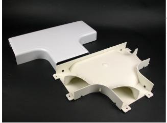
A full capacity tee fitting for branching raceway at right angles. Provides separation of services and 2'' (51mm) cable bend radius for UTP and Fiber Optic installations.
