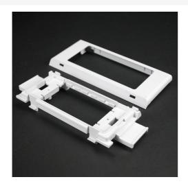
For power or communication devices in a single compartment. For use with 5507 Series Faceplates, Ortronics TracJack and Series II Modules, Pass and Seymour Activate Series Inserts, and Wiremold Open System Communication Modules. NOTE: CM-EPLA End Plates are required when using Wiremold communication modules and Pass and Seymour Activate inserts. S2-EPL End Plates are required when using Orthonics Series II Inserts. To mount TracJack inserts, use 5507-4TJ or 5507-6TJ Faceplates.
