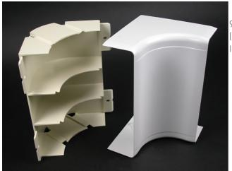
90 degree internal corner, with integral dividers, that provides a 2'' (51mm) cable bend radius for UTP and fiber optic installations. Ideal for lay-in or pull-through installations.
