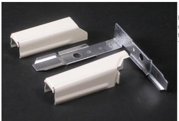
For 90 degree twist with a 90 degree turn. For double turn at right angles from one surface to another. For transitions from a sidewall to ceiling or edge of door or window trim. Twistout in cover adapts for use with 700 Series Raceway.
