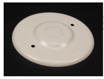
1/2" trade size KO in center. For use with 5735, 5737, 5737A, 5738, 5738AF, 5739, 5739A, or 2135 Device Boxes. Converts these boxes into pull or junction boxes for hanging lightweight pendant fixtures with 1/2" trade size pipe stems.
