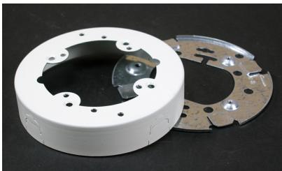
Mounts onto 3 1/4" or 4" (83mm or 102mm) conduit boxex, or other recessed outlets. Cover accepts devices with mounting screw centers of 2 3/4", 3 1/2", or 4 1/16" (70mm, 89mm, or 103mm). Can be used with 5736 Blank Cover as a pull or junction box. Outside diameter 4 3/4" (121mm).
