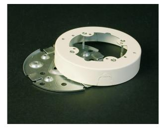
Cover accepts fan bracket device with mounting centers of 3 3/16" (81mm). Base has six mounting holes and 4 1/2" trade size KOs. #10 mounting studs provided. Rated for fans and fixtures up to 50 lbs. NOTE: Certified to Canadian Safety Standards for sale in Canada. When ordering these products, change the "V" color prefix to "vc" or the "WH" color suffix to "WHC" to denote the Canadian versions.
