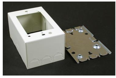
Designed especially for use in the installation of signal system and alarm wiring. Base has 1/2" trade size KOs. Larger gang boxes available by special order. Single-gang: 4 5/8" L x 2 7/8" W (117mm x 73mm). Accepts NEMA single-gang standard faceplates. NOTE: Certified to Canadian Safety Standards for sale in Canada. When ordering these products, change the "V" color prefix to "vc" or the "WH" color suffix to "WHC" to denote the Canadian versions.
