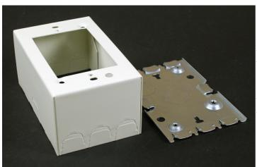
For deep devices such as momentary contact, remote control switches, and hospital signaling system devices. Base has 1/2" trade size KOs. Larger gang boxes available by special order. Single-gang: 4 5/8" L x 2 7/8" W (117mm x 73mm). Accepts NEMA single-gang standard faceplates. NOTE: Certified to Canadian Safety Standards for sale in Canada. When ordering these products, change the "V" color prefix to "vc" or the "WH" color suffix to "WHC" to denote the Canadian versions.
