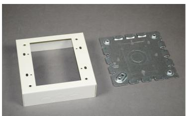
For standard shallow switches and receptacles including single-gang combination devices. Base has two 1/2" trade size KOs. Larger gang boxes available by special order. Two-gang: 4 3/4" L x 4 3/4" W (121mm x 121mm). Accepts NEMA double-gang standard faceplates. NOTE: Certified to Canadian Safety Standards for sale in Canada. When ordering these products, change the "V" color prefix to "vc" or the "WH" color suffix to "WHC" to denote the Canadian versions.
