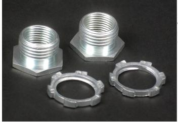
For hanging either 3/8"" (9.5mm) or 1/2"" (12.7mm) fixtures to Wiremold fittings with 1/2"" trade size KOs. Has female 3/8"" (9.5mm) pipe thread inside and male 1/2"" (12.7mm) pipe thread outside.
