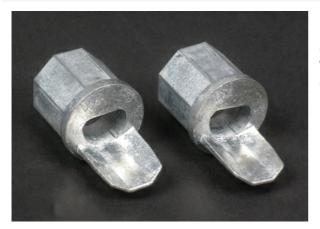
Interior threaded female connector with a 1/2inch trade size conduit opening for connecting Wiremold 500/700 Series raceway to conduit. When used with 700 Series Raceway, break out crescent twistout in connector.
