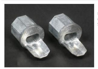
Interior threaded female connector with a 3/4" trade size conduit opening for connecting raceway to conduit. When used with 700 Series Raceway, break out crescent twistout in connector.
