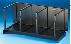
Ortronics bend limiting cable management panels have curved falls that protect against cable crimping and also maintain proper bend radius. 7" H x 7" D rings with waterfall, 8.34" H x 19" W, 4 rack units, black.
