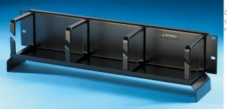
Ortronics bend limiting cable management panels have curved falls that protect against cable crimping and also maintain proper bend radius. The panels are ideal at the top of standard 19" EIA racks. 3.5"H x 3.5"D rings with waterfall, 2 rack units, black.
