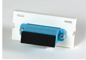
The Series II, Multimode, SC Duplex, Aqua Adapters (2-Fiber), White Adapter Plate, has one duplex adapter with 180° exit, and ceramic alignment sleeves. This adapter panel is 1 unit high. These adapter panels include dust caps, and offers two insests for optional icons (Not Included), to label each connector and indicate its purpose. Compatible With: Series-II Workstation Face Plates and Series-II Workstation Surface Mount Boxes. Wiremold raceway series 2700, 2800, and 2900
