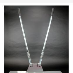
Portable cutter for 3000 Series Raceway Base. Provides clean and easy square cuts.  $\,$
