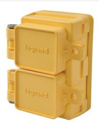
Turnlok Watertight Duplex Receptacle, 15amp 250volt, NEMA Configuration L6-15, Impact resistant Valox lid, cover plate, and receptacle body withstand impacts, chemical, and corrosion.
