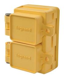
Turnlok Watertight Duplex Receptacle, 15amp 250volt, NEMA Configuration L6-15, Impact resistant Valox lid, cover plate, and receptacle body withstand impacts, chemical, and corrosion.
