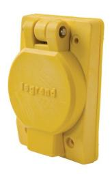
Turnlok Watertight Single Receptacle, 20amp 125/250 volt, NEMA Configuration L14-20, Impact resistant Valox lid, cover plate, and receptacle body withstand impacts, chemical, and corrosion.
