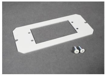
Used for floor coverings greater than 5/16'' (7.9mm). The 6TS will allow the top surface of the cover to be flush with the finished floor. Includes six (6) 1/16'' (1.6mm) thick shims. Up to a total of 3/8'' (9.5mm) of adjustment.
