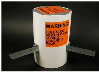
Nonmetallic sleeve attaches to structural decking and maintains 6inch - 6 1/8inch diameter cast in hole. Unit includes three (3) attachment legs, two (2) end caps and three (3) thumb screws.
