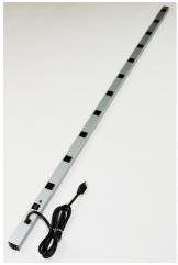
Eleven outlets. 6' (1.8m) cord. Length 70"" (1.8m). 15A resettable circuit breaker. Computer grade surge protection, 15 Amps.
