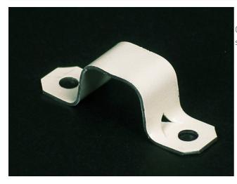
Converts to one hole by breaking off at score. Lanced tab holds strap in place while fastening to surface.
