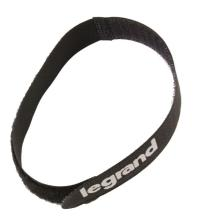
Cable management straps provide an organized solution for the management of patch and horizontal distribution cables. The 3/4 in W straps have a hook and loop type closure to secure and administer cables without damaging the construction of the copper or fiber cable.
