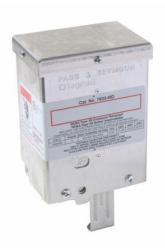
Three pole, Three Phase AC Manual Motor Controller 30 amp, 600 watts., Suitable as Motor Disconnect - 10KA @ 600VAC, 30A max Class J fuse.
