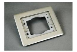
One-gang powder-coated aluminum combination carpet and tile flange, 6'' x 5'' (152.4mm x 127mm). Accepts Ortronics MAB6TJ TracJack and MAB3S2 Series II adapters and Wiremold CM Series Open System inserts, sold separately. NOTE: UL Listed for tile, terrazzo, and carpet floors. Brass covers and flanges are not interchangeable with aluminum or nonmetallic covers and flanges. Nonmetallic covers are interchangeable with aluminum flanges.
