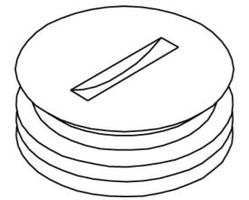
1/2" (12.7mm) diameter brass abandon plug. Thread size is pipe thread size.
