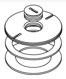
Brass conversion kit which includes one 825A-1/2; 1/2" (12.7mm) diameter plug, one 825C-1/2, one 825L, and one 825N. For carpet or tile installations.
