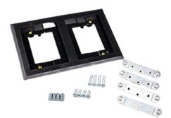
Two-gang nonmetallic carpet flange. For Ortronics connectivity use with 829PFLRT Cover. For Wiremold Open System connectivity use with 829PFL Cover. Accepts Ortronics MAB6TJ TracJack, MAB3S2 Series II and Wiremold CM Series Open System adapters, sold separately. NOTE: Polycarbonate cover plates can only be used with polycarbonate flanges.
