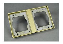
Two-gang powder-coated aluminum tile flange, 4 1/2" x 7 5/8" (114mm x 194mm). For use on 880S2, 880M2, 880CS2-1, and 880M2-1 Floor Boxes. NOTE: UL Listed for tile, terrazzo, and carpet floors. Brass covers and flanges are not interchangeable with aluminum or nonmetallic covers and flanges. Nonmetallic covers are interchangeable with aluminum flanges. Made in USA.
