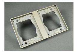
Two-gang powder-coated aluminum tile flange, 4 1/2" x 7 5/8" (114mm x 194mm). For use on 880S2, 880M2, 880CS2-1, and 880M2-1 Floor Boxes. NOTE: UL Listed for tile, terrazzo, and carpet floors. Brass covers and flanges are not interchangeable with aluminum or nonmetallic covers and flanges. Nonmetallic covers are interchangeable with aluminum flanges. Made in USA.
