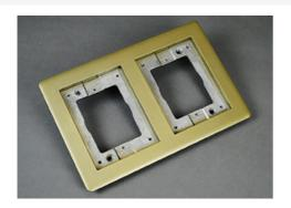
Two-gang powder-coated aluminum combination carpet and tile flange, 6" x 9" [152.4mm x 228.6mm]. Accepts Ortronics MAB6TJ TracJack and MAB3S2 Series II adapters and Wiremold CM Series Open System inserts, sold separately. NOTE: UL Listed for tile, terrazzo, and carpet floors. Brass covers and flanges are not interchangeable with aluminum or nonmetallic covers and flanges. Nonmetallic covers are interchangeable with aluminum flanges.
