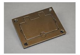
Brushed aluminum GFI cover plate, 3.290'' x 4.310'' (83.6mm x 109.5mm). May be used with Wiremold CM Series adapters and Ortronics Connectivity Systems in conjunction with 817B, 827B, and 837B Flanges. Made in USA.
