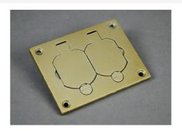
Brushed aluminum duplex cover plate, 3.290" x 4.310" (83.6mm x 109.5mm). Flip lids can also be used with 106 type frames for communications. NOTE: Brass covers and flanges are not interchangeable with aluminum or nonmetallic covers and flanges. Nonmetallic covers are interchangeable with aluminum flanges. Made in USA.
