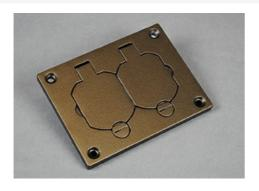
Brushed aluminum duplex cover plate, 3.290" x 4.310" (83.6mm x 109.5mm). Flip lids can also be used with 106 type frames for communications. NOTE: Brass covers and flanges are not interchangeable with aluminum or nonmetallic covers and flanges. Nonmetallic covers are interchangeable with aluminum flanges. Made in USA.
