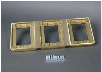
Three-gang brass (837T) tile flange. For use on 880S3, 880M3, 880CS3-1, and 880CM3-1 Floor Boxes. NOTE: Brass covers and flanges are not interchangeable with aluminum or nonmetallic covers and flanges. Nonmetallic covers are interchangeable with aluminum flanges.
