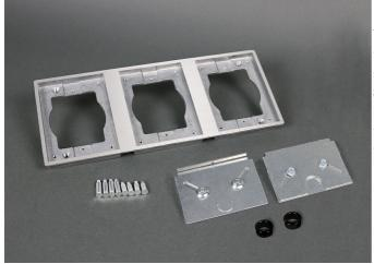
The 838TAL-880 Series Flanges provide additional load support for 3-gang tile flanges. Kit includes 838TAL Flange, and two support dividers. Order kit for specific box type: 880S3, 880M3, 880CS3, or 880CM3. NOTE: Brass covers and flanges are not interchangeable with aluminum or nonmetallic covers and flanges. Nonmetallic covers are interchangeable with aluminum flanges.
