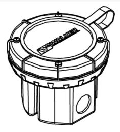
Die-cast aluminum construction with three 1/2"" (12.7mm) knockouts, two on the sides and one on the bottom. 18 cu. in. (295ml3) of capacity. Requires a 4"" (102mm) diameter hole. Comes complete with a disposable cover, receptacle and cover sold separately.
