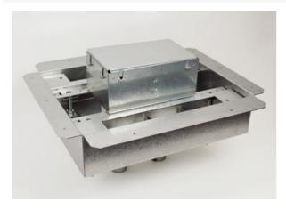
2-Gang Fire Classified Steel Floor Box. Adjustment range over deck of 2" (51mm) minimum to 6-1/2" (165mm) maximum. One 1 1/4" (32mm)and One 2" (51mm) conduit feed openings. Box Capacity - 58.5 cubic inches each gang. This floor box preserves up to a 3-hour fire rating of floors in which it has been installed.
